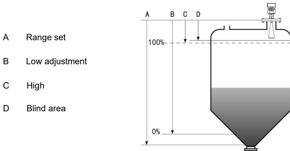
**Datum measurement:** Screw thread bottom or the sealing surface of the flange.
