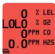
Red display in alarm conditions
