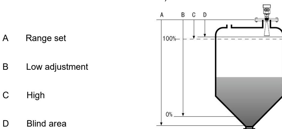
Datum measurement: Screw thread bottom or the sealing surface of the flange.
